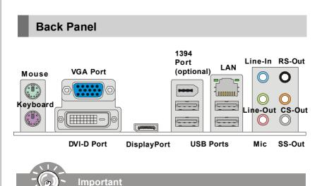
When there is any expansion card inserted in the PCIE x16 slot, the VGA, DisplayPort and DVI-D port will not output any signal.
